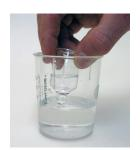
Fill a 10-ml sample cell with sample and cap the cell. This will be the sample cell blank. Wipe excess liquid and fingerprints from the sample cell blank.
