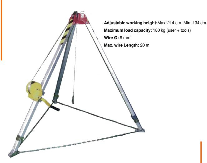
It incorporates an automatic block winch rescue which can be placed on top of the tripod or in one of the feet.
