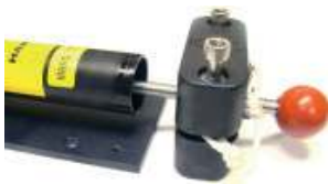
2. Remove lower bracket and take out the piston rod.
