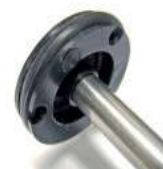
4. Apply a layer of new lubricant to the O-ring and piston recess. Put the O-ring back in position and apply a thin layer of lubricant to the outside of the O-ring.
