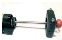
2. Remove lower bracket and take out the piston rod.
