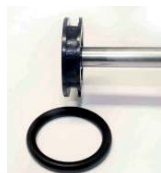
3. Remove the O-ring from the piston with a blunt tool. Do not damage the O-ring or the piston. Clean the O-ring and the piston recess.
