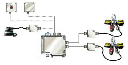
HM-0460 Outputs: 2 Inputs: 1 Backup-battery: Up to 24 hours operating time
