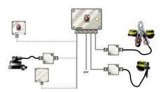
Release switch - RS Remote release system for one liferaft
